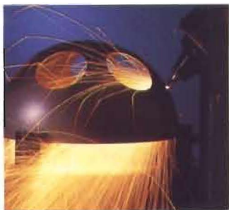
Laser cutting holes in hydroformed hemisphere. Hole size and location are programmed on off-line programming system.
