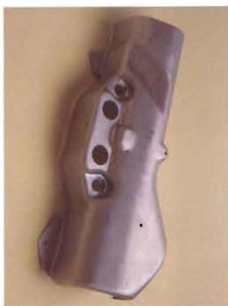
Laser trimmed and cut formed stainless steel part. The cut path is generated through a combination of TEACH mode (for border trim) and on-line programming (holes).
